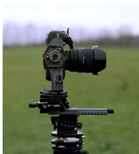
Figure 2. 35mm camera on a segmented panorama tripod head, viewed from the side. Photo by Tom Watson.
