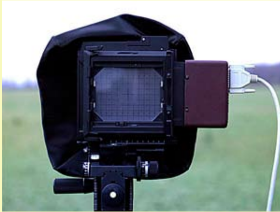
Figures 9-11. Better Light with the view camera shifted to the left, right and center. The combination of left and right make a rectilinear panorama image. Photos by Tom Watson.
