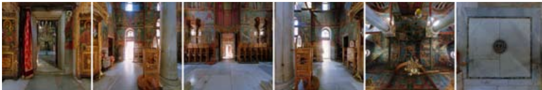
Figure 4. Six rectilinear cube faces (90° by 90° each) derived from the equirectangular image in Figure 3.
