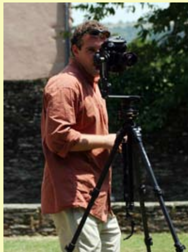
Figure 12. Michael Gross in the cloister of the Sainte Foy Abbey Church in Conques, France (1050-1120). The system used consists of a Canon 1Ds Mark II (16.7MP digital full-frame SLR), Canon Wide Angle EF 14mm lens, Bogen/Manfrotto 303SPH Spherical Panorama Tripod Head, Bogen/Manfrotto 055MF4 Magfiber Tripod, and Canon Remote Switch. Photo by Barry Gross.
