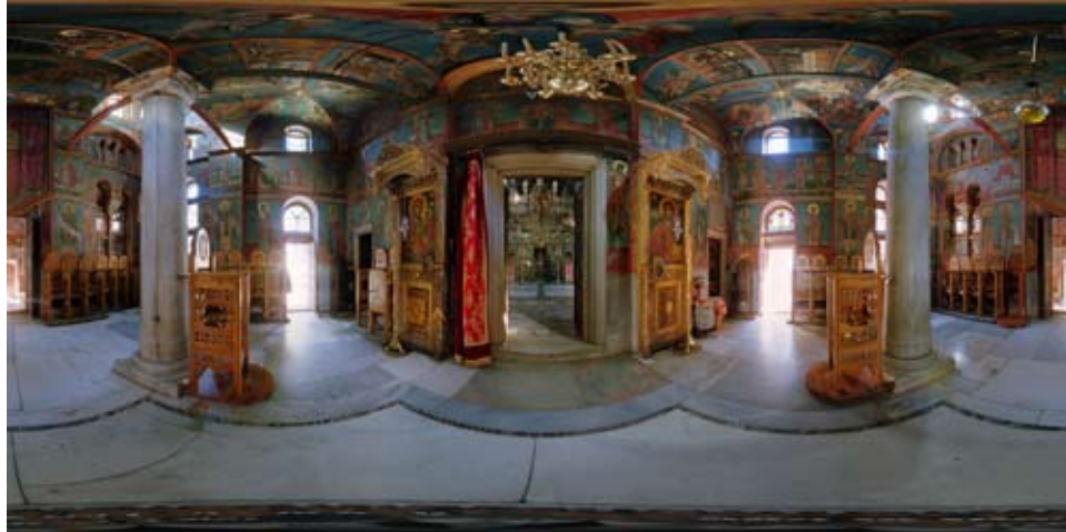
Figure 3. Equirectangular projection, 180° vertical field of view.
