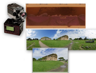
Figure 1. Seitz 220VR rotational film camera. Top to bottom, example of a negative, spanning 410^\circ degrees, from Seitz camera (using 20mm lens). Positive after scanning, and cropping to 360^\circ degrees. The cylindrical perspective results from the use of a rotational camera.
