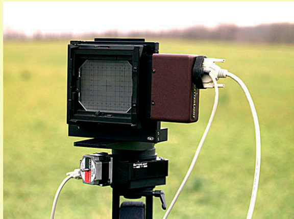
Figure 8. Better Light scan back mounted on a Better Light Panowide adapter. Photo by Tom Watson.
