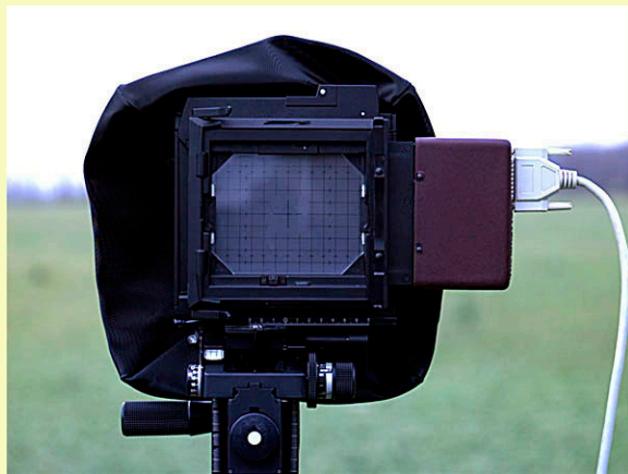
Figures 9-10. Better Light with the view camera shifted to the left and right. The combination of left and right make a rectilinear panorama image. Photos by Tom Watson.
