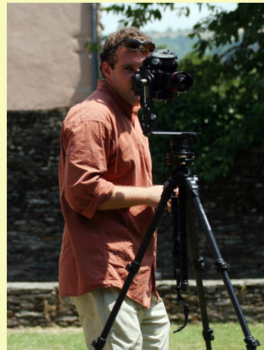
Figure 11. Michael Gross in the cloister of the Sainte Foy Abbey Church in Conques, France (1050-1120). The system used consists of a Canon 1Ds Mark II (16.7MP digital full-frame SLR), Canon Wide Angle EF 14mm lens, Bogen/Manfrotto 303SPH Spherical Panorama Tripod Head, Bogen/Manfrotto 055MF4 Magfiber Tripod, and Canon Remote Switch. Photo by Barry Gross.
